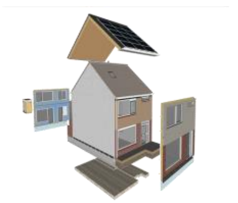
Figure 32: holistic systemic deep renovation concept- Rennovates
