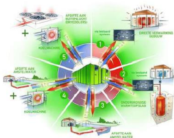
Figure 52: Innovative solutions applied to Amsterdam’s own public data centres- use of an existing Aquifer Thermal Energy Storage (ATES)
