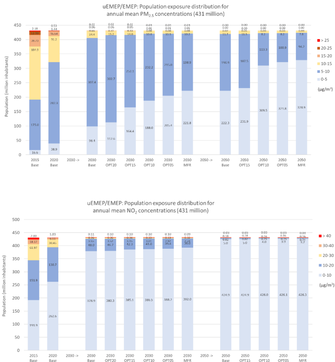
Figure A5.21 – Number of people exposed above selected annual mean concentrations in the EU-27 for PM 2.5 and NO 2
