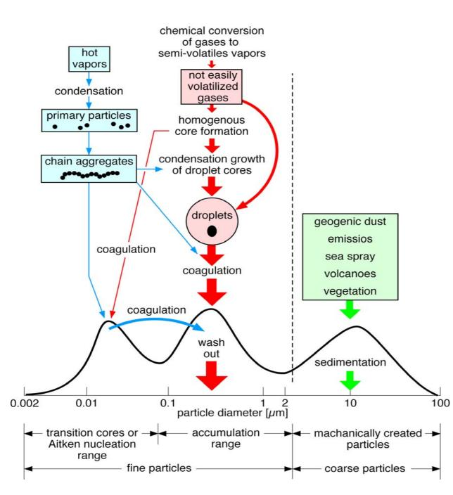
Formation of fine and ultrafine Particles: 2 different Mechanismes
