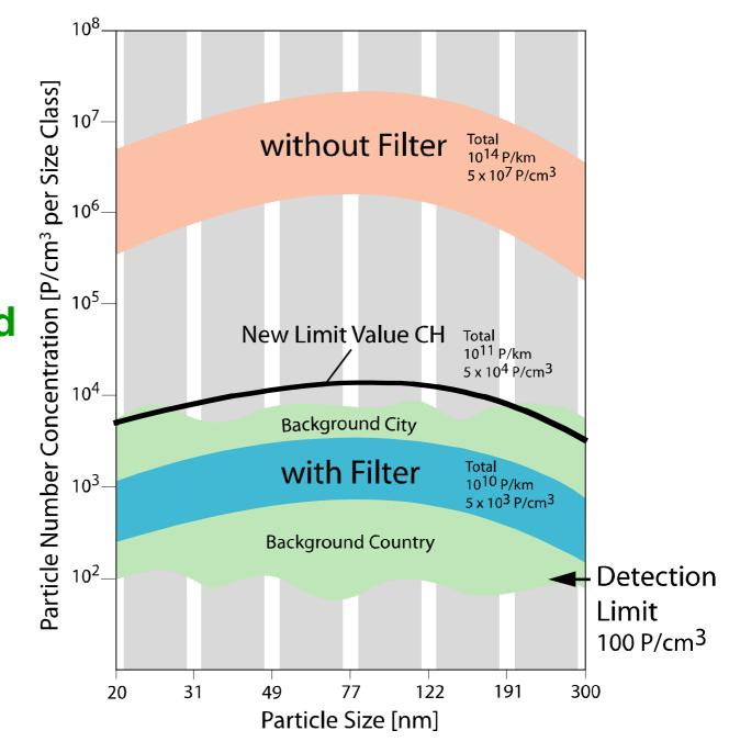
Exhaust Gas downstream of the Filter is cleaner than Ambient Air !
