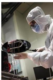
An operator handling a 300mm silicon wafer in a clean room, Grenoble, France, 4 February 2022.
