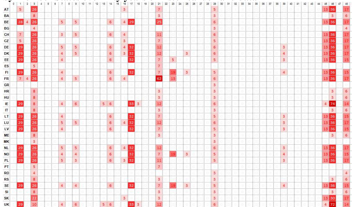
Graph 2: Distribution of prices at VoLL in the context of a well-integrated market by Member States over fifty years of historical demand data
