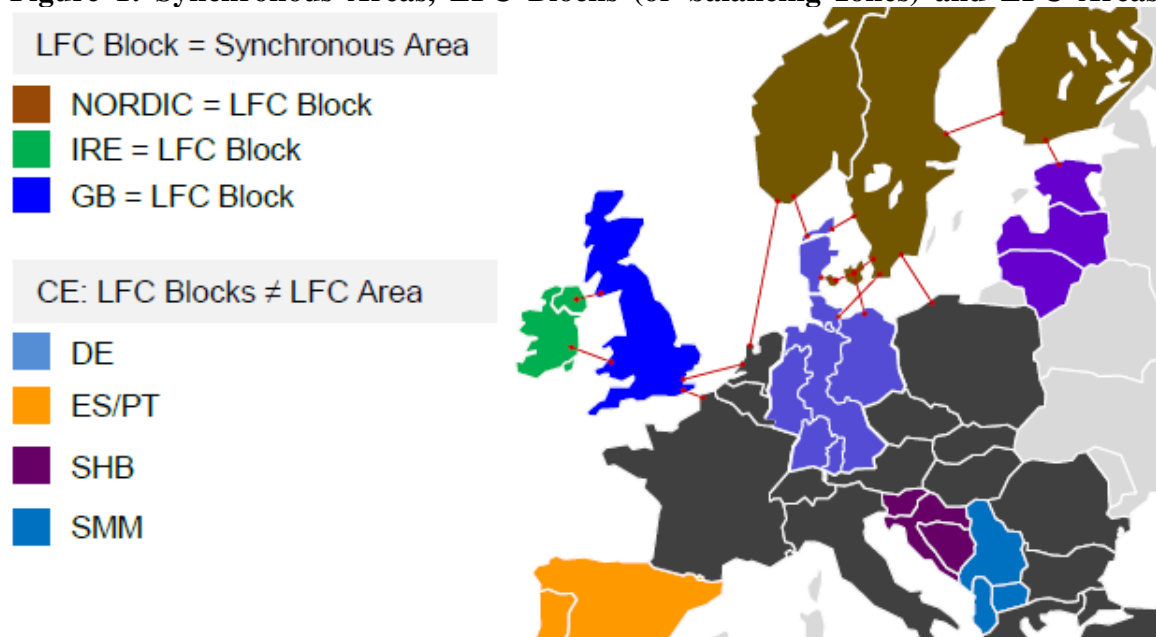
Figure 1: Synchronous Areas, LFC Blocks (or balancing zones) and LFC Areas
