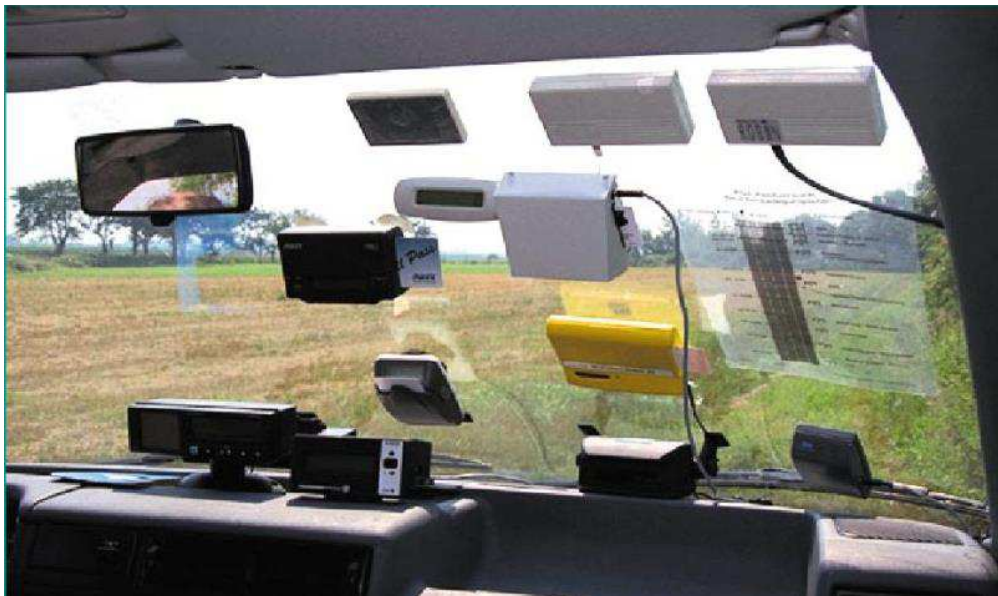
Figure 1: A lorry equipped with the different OBUs needed to drive unhindered on EU roads. Source: 4icom, Steer Davies Gleave, op. cit. footnote 17
